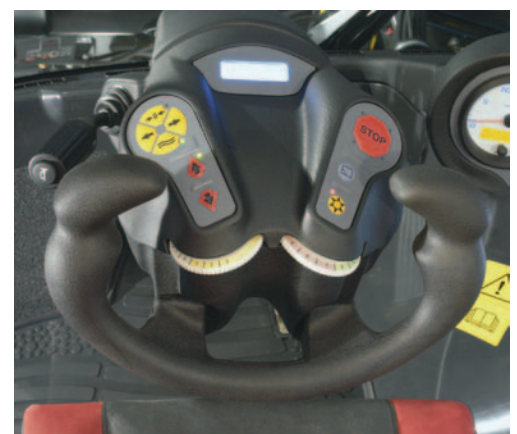
Half-cut airplane-style steering wheel with built-in multifunctional display
