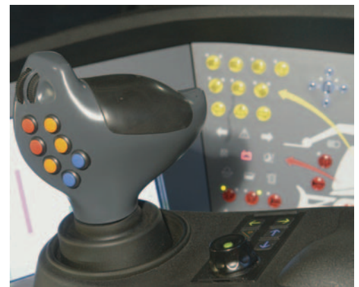
Ergonomic joystick for the driver to simply rest his hand on. All switches and indicator lights are color-coded for the various operations and functions.
